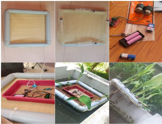
Fig.2 Construction of Automated Floating Island
